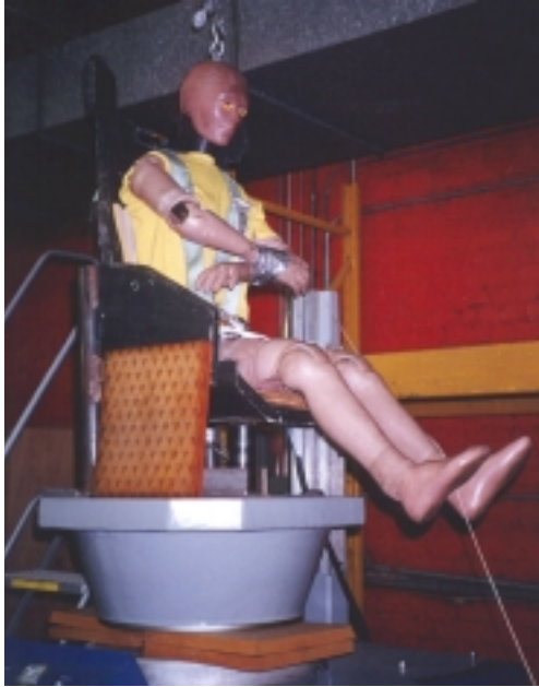
Figure 5. Hybrid III Female Mannequin in Cobra Impact Test System
